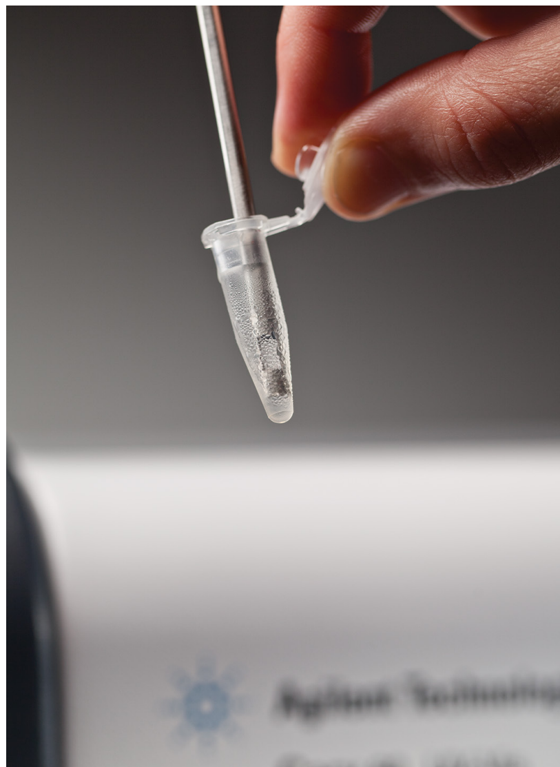
Figure 6. A fiber-optic probe accessory can be fitted to a UV-Vis spectrophotometer to measure liquid samples in a range of containers.
