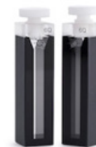
Figure 20. A 10 mm pathlength, 1.4 mL volume semi-micro cell.
