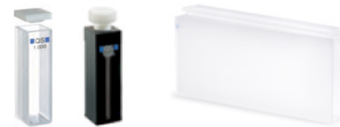
Figure 15. Cuvettes for measuring liquid samples. From left to right: A standard 10 mm pathlength, 3 mL cuvette, an ultramicro cell for measuring very low volumes, and a long pathlength cuvette for dilute solutions.
